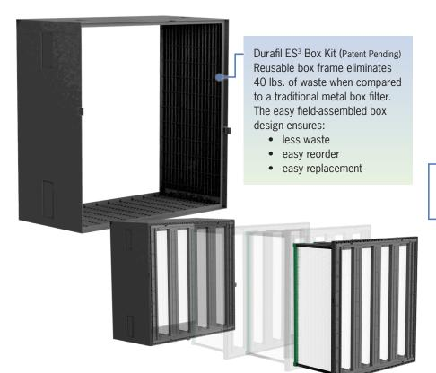
Built-in prefilter spacer section that eliminates an unnecessary blockage of airflow common in other V-style filters when a prefilter is mounted directly to the face. This engineered feature on the ES<sup>3</sup> reduces pressure drop and saves energy costs of approximately \$50 per filter per year.
